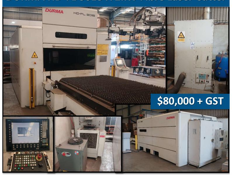
Made in Turkey – YR 2013 • X Axis - 3060mm, Y Axis - 1530mm, Y Axis – 160mm • 2kW IPG Laser Source • Precitec Head • Max. Sheet Size - 3048mm x 1524mm • Max. Cutting Speed: 200m/min • Max. Acceleration: 20m/s² • Lantek Nesting Software • Twin Change Tables
