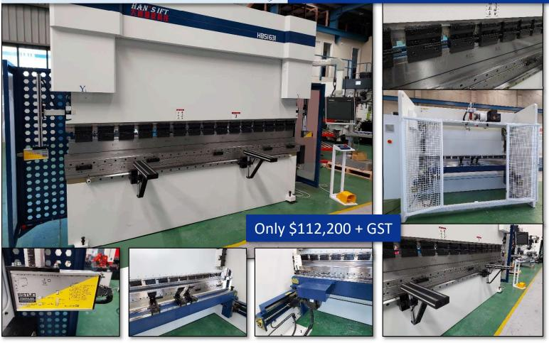
The HAN's HBS1631 Press Brake is your high accuracy, simple operation, economical metal bending solution. With 5-Axis (Y1, Y2, X, R, Crowning) and FAGOR brand optical grating scales to measure the position of the moving rams. Fiessler light safety system following top tool, sheetmetal guards on sides and rear gate, all with microswitch interlocks and emergency stop foot pedal. Our stock HSB1631 machine includes a DELEM 15" touchscreen controller and Euro style quick release top tool clamps.
