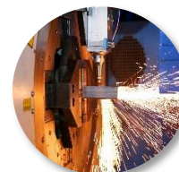
Tip nozzle cutting head
