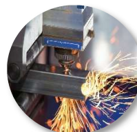
Standard laser cutting head
